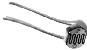
Figure 11 – Photo of the small cadmium sulfide photoconductor cell of the type used in this compressor circuit. It has a diameter of about six millimeters.
