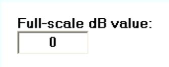
This defaults to zero but other values can be entered. For example a vu meter would have an entry of "3" in this box; this would set the full-scale value to +3 dB.
