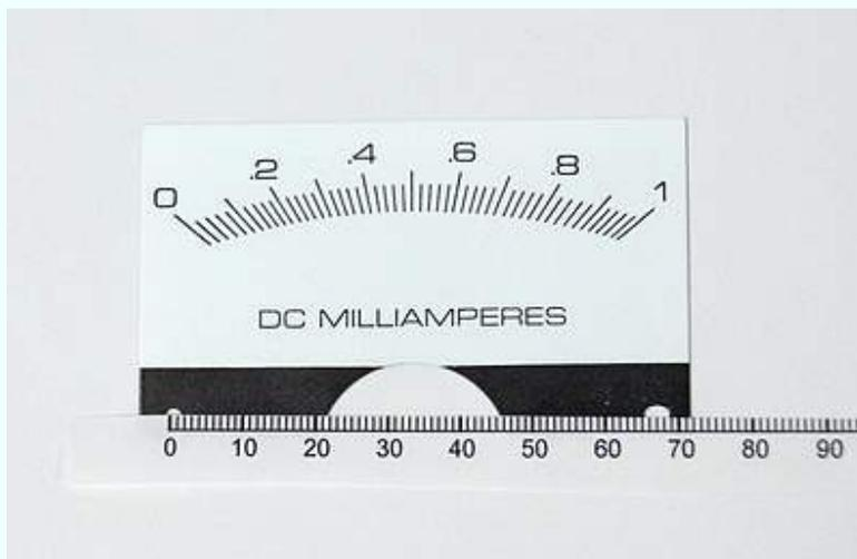
Now measure the separation between the mounting holes (67 mm here). **This must be an accurate measurement.**
