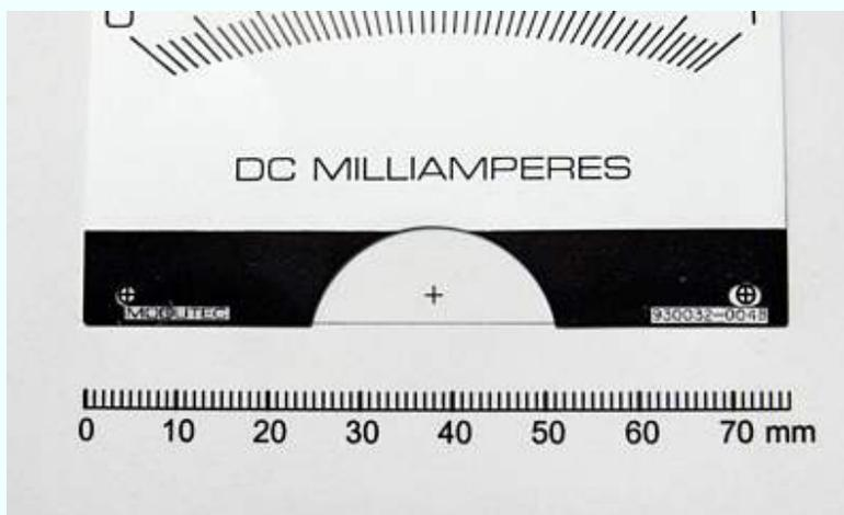
Print a scale and confirm that the mounting hole separation is correct, as shown here by laying the plate on top of the printout.
