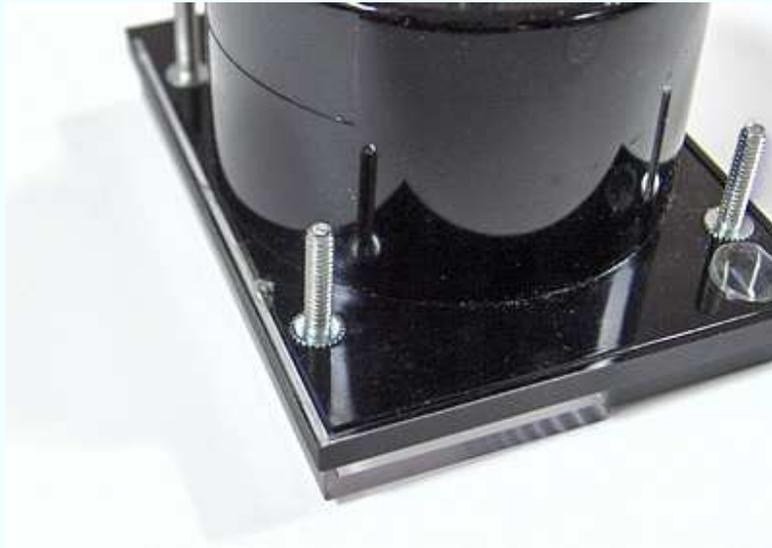
Open the case to access the plate on which the scale is printed. Here we see that perhaps some glue is used to seal the case. Carefully break the seal or otherwise open the case. For those cases that are held together with screws simply unscrew them.
