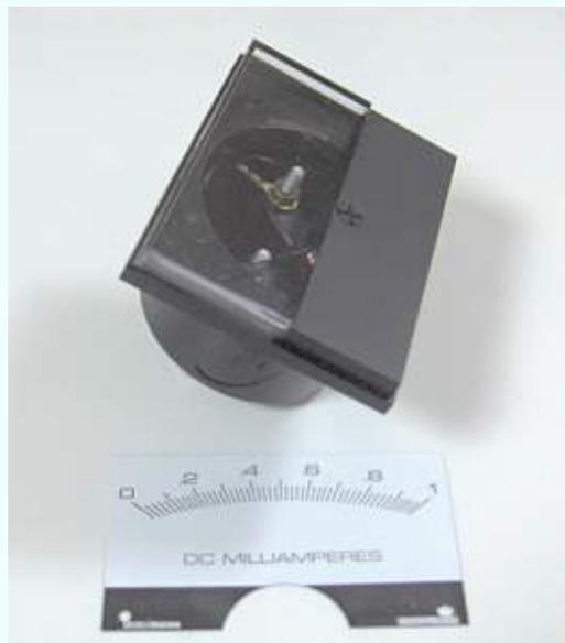
Place the front cover back on the case so that the interior portion of the meter will be kept clean.
