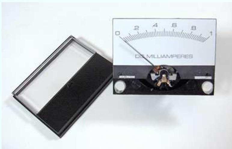
Remove the face (front) of the assembly and set it aside.
