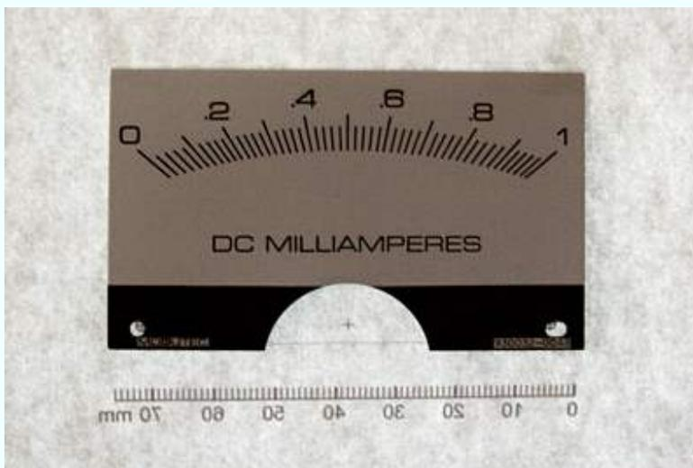
Place the *reverse* side of the metal plate against the non-printed side of the newly-printed scale. (By doing this, the original lettering will not show through the new paper scale.)
