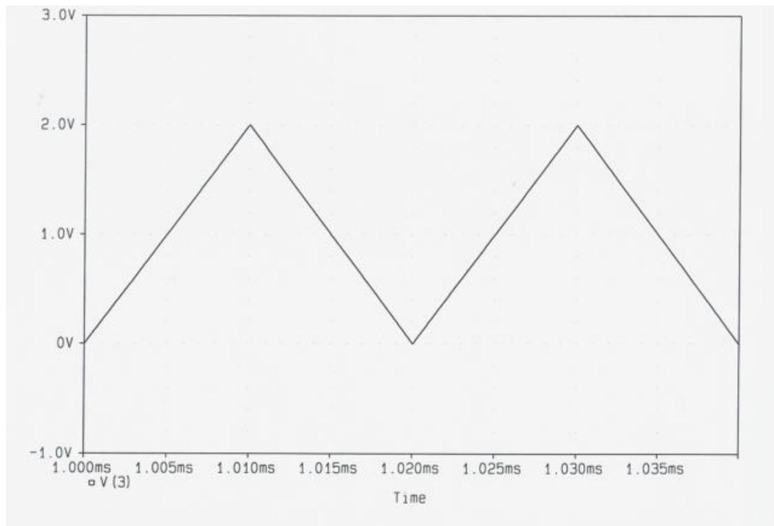
This should be considered a well-behaved triangular wave. It is in fact difficult to generate and for this reason an integrated circuit designed specifically to produce such a signal is commonly used. There may be a temptation to use a squarewave followed by a simple waveshaping network in an attempt to generate the triangular wave.
