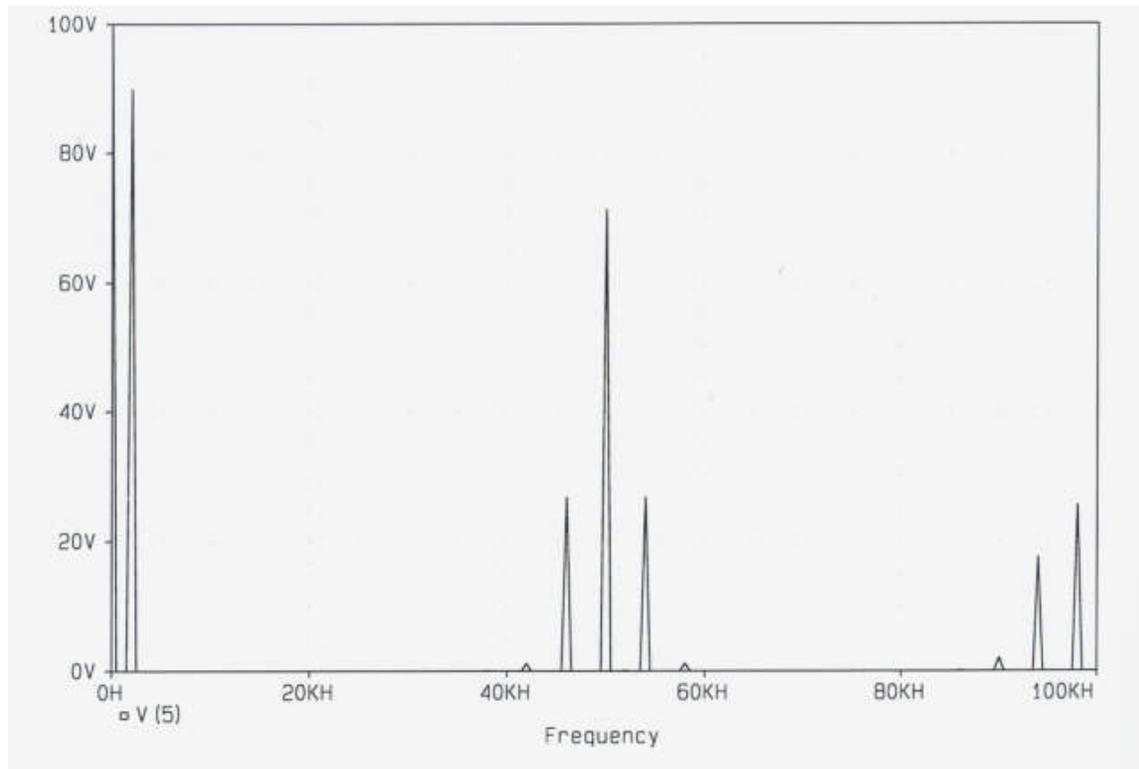
Here we see at 0 Hz 100 volts of DC corresponding to the idling carrier level. We can see 90 volts of a modulating signal at 2000 Hz.
