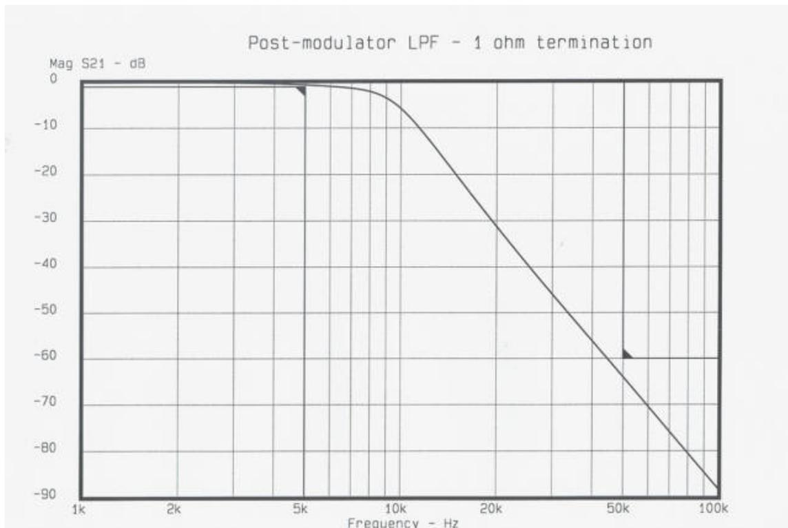
This filter will pass the DC and audio components while satisfactorily rejecting the switching signal components.
