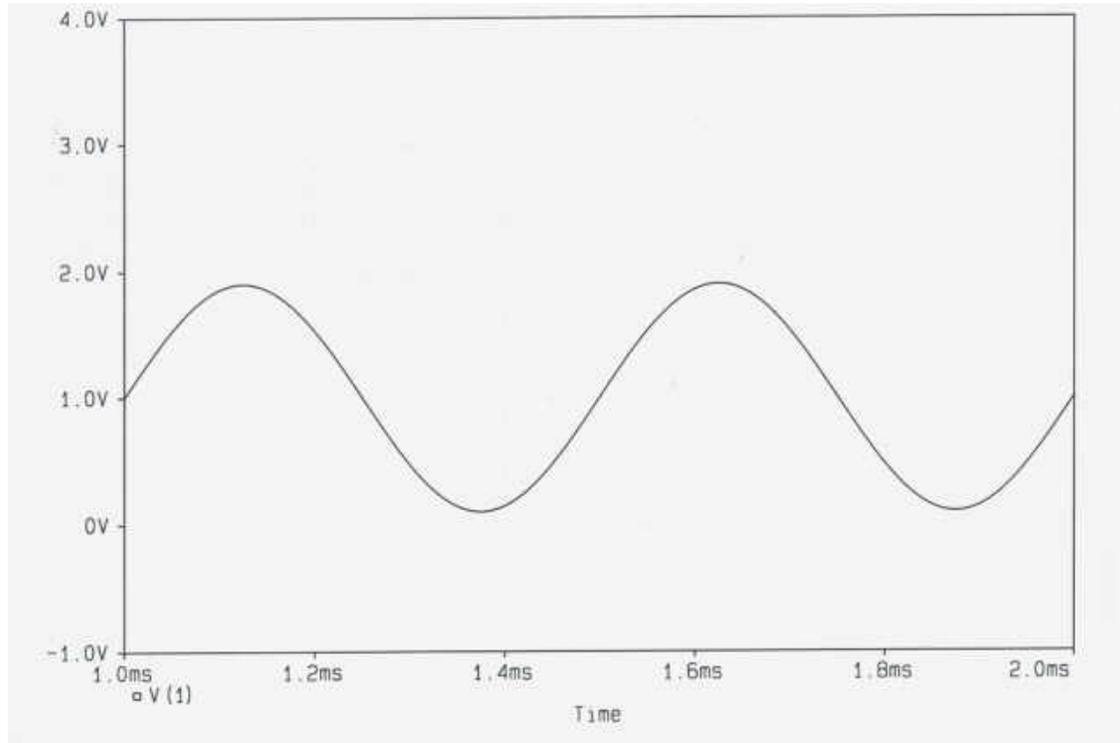
This waveform consists of two components. One is a DC signal corresponding to the carrier level and the other is the modulating sinusoid itself, set here to a frequency of 2000 Hz. The DC level has been set to 1.0 and the peak amplitude of the sinusoid has been set to 0.9, corresponding to 90% modulation.
