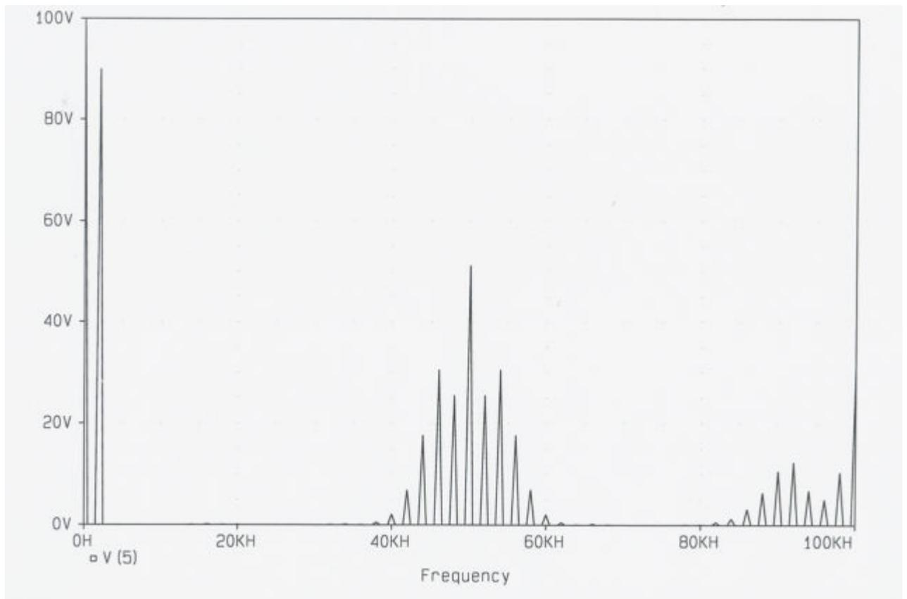
Either commparison waveform (triangle or sawtooth) should work well.
