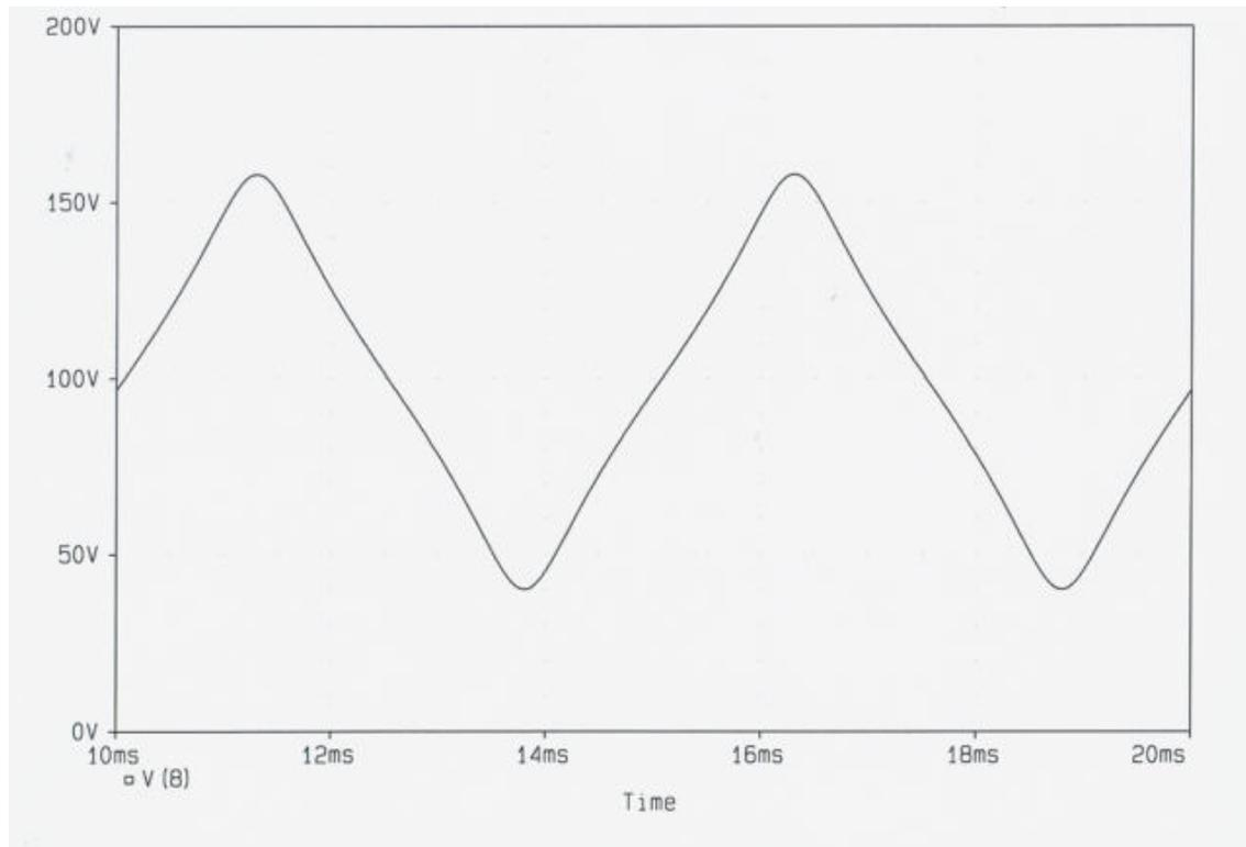
Analysis of this obviously defective sinusoid reveals a significant harmonic content. The waveform shows that its peaks are stretched slightly. A more palatable distortion would be to have the peaks compressed a small amount. Further, the overall amplitude has been reduced with this defective triangle comparison wave..
