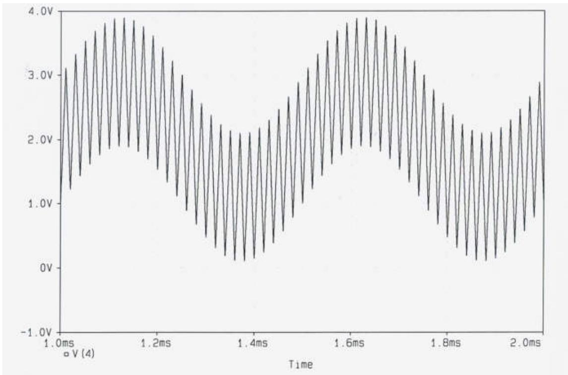
This signal is applied to a comparator which (in this case) generates an output when the sum exceeds 2 volts and generates no output when the sum is less than 2 volts. The output we are referring to here has been set to a value of 200 volts. This makes it easy to think in terms of "modulation percentage."
