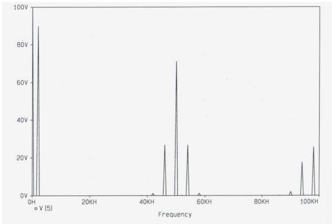
Here we see the switcher output spectrum in a system using a *sawtooth* comparison signal:
