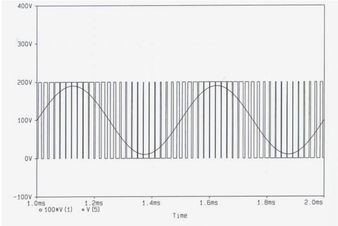
The modulating waveform has been superimposed on the comparator output to allow a simple comparison of the instantaneous value of the modulating waveform with the output of the comparator. As the modulating waveform value increases the duty cycle of the comparator output also increases.
