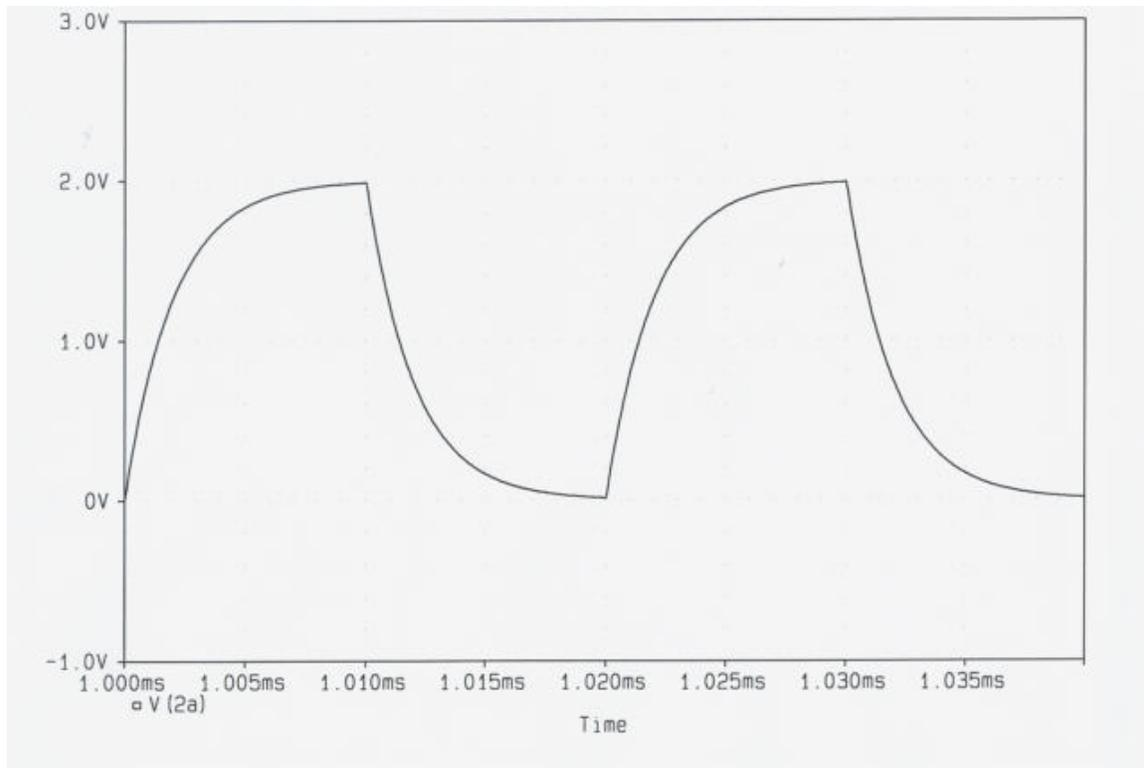
If that poor triangular waveform is used as the comparison wave to generate our PWM signal we will see the following final signal from the output lowpass filter, a modulator output which is obviously quite substandard:
