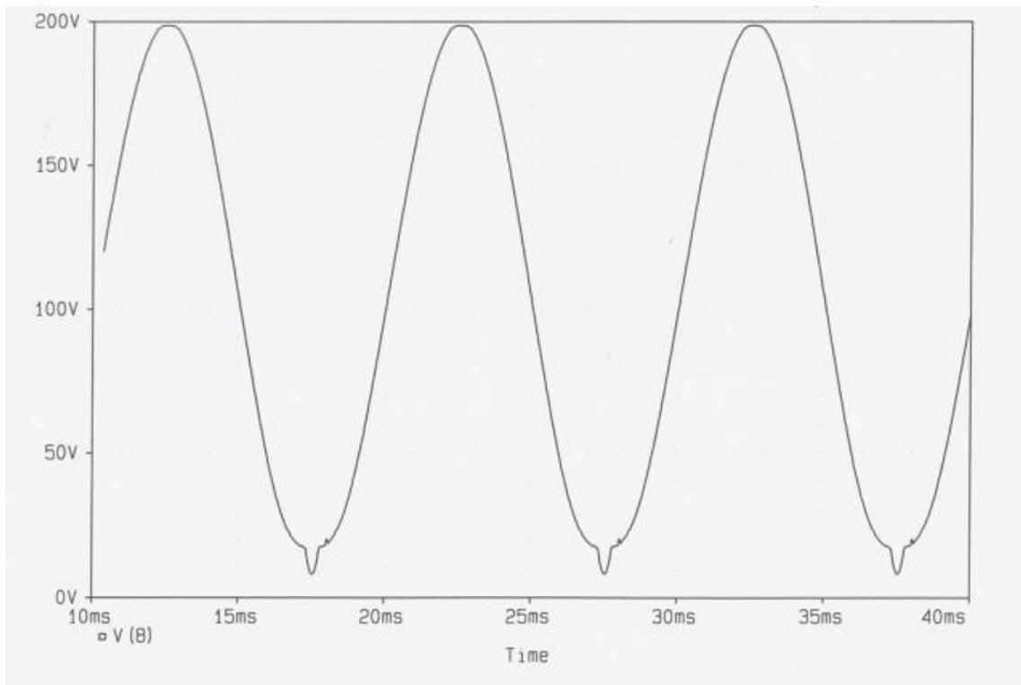
If the capacitance to ground from this node is appreciable, the switcher may charge that small capacitance in a single cycle but the capacitance can discharge only through the remainder of the filter into the output load. The result is serious distortion of the modulation envelope on the negative peaks ("troughs").
