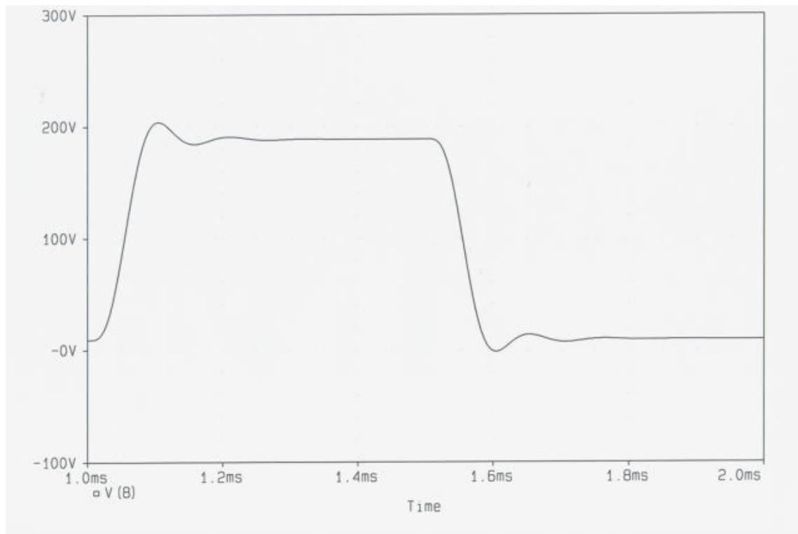
The post-modulator lowpass filter is the only item contributing to alteration of the modulating waveform. The overshoot seen here, which is quite modest and acceptable, is due entirely to the filter. Rephrased, the filter alone has an identical effect on the modulating waveform.
