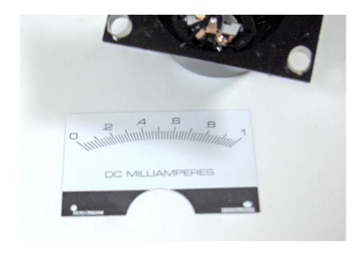
Figure 5 shows the plate separated from the meter case.
