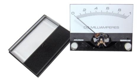
Figure 2 shows that we are to remove the face (front) of the assembly and set it aside.
