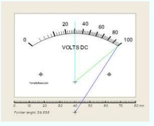
Adjusting the exponent upward, to over 1.0, can make the scale of a rectifier-type AC voltmeter be correct. The scale below is an example of adjusting the exponent to 1.3 to simulate a noticeably nonlinear AC voltmeter scale. As in the case of the wattmeter, the value of the exponent can be adjusted to maximize accuracy in a given case.
