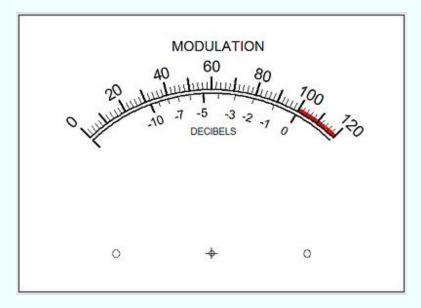
Now let us apply a correction. This might be for a nonlinear meter movement or for a nonlinear driving electronics circuit. In this case we have applied a nonlinearity in the low-current area, such as might be encountered in a semiconductor diode rectifier.
